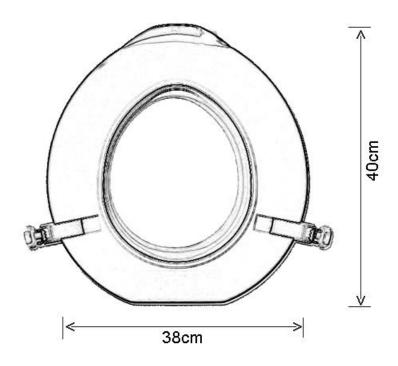
Brackets adjust to suit toilet bowls between 315mm minimum to 370mm maximum width.
